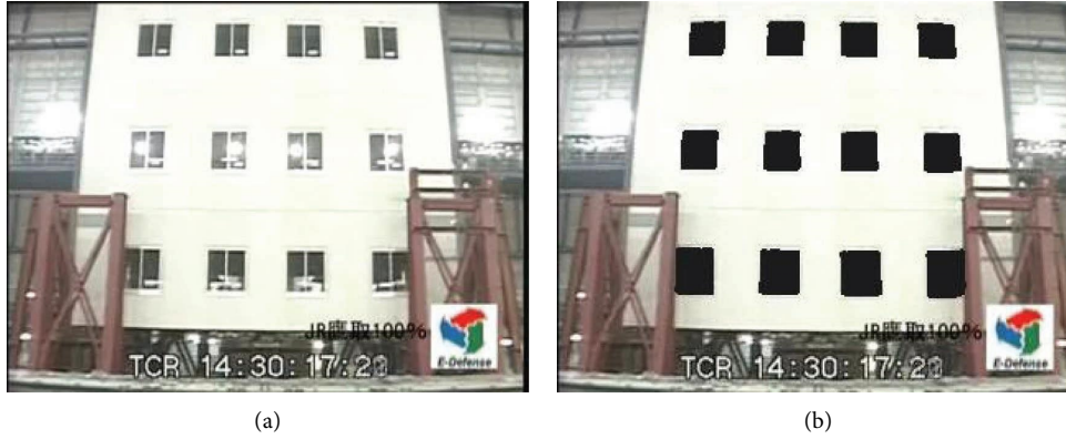
FIGURE 4: An example of structural RoU identification based on TL. (a) Before RoU (original frame). (b) After RoU (processed frame).
