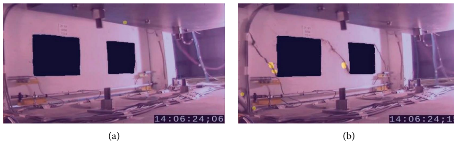
FIGURE 11: Results of feature enhancement for the pronounced shear cracks (derived to differentiated continuous frames around t = 4.2 s in (a) and t = 4.5 s in (b)). (a) Before crack occurrence. (b) After crack occurrence.
